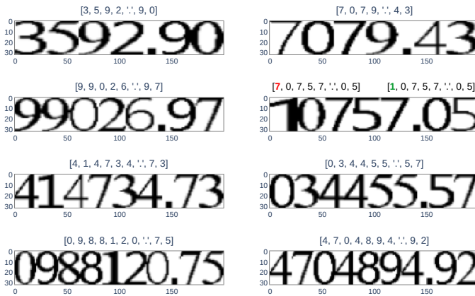
FIGURE 7. Results of recognition of cadastral coordinates. One of the coordinates was recognized with an error
