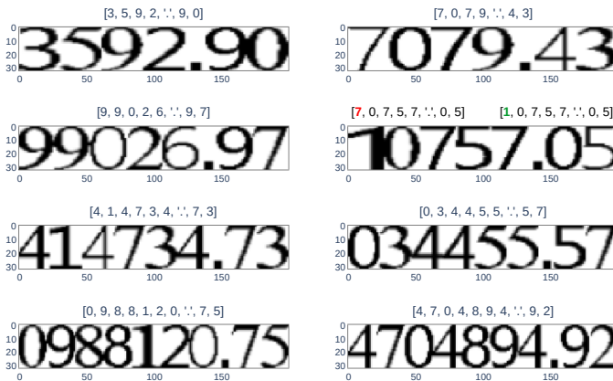
FIGURE 7. Results of recognition of cadastral coordinates. One of the coordinates was recognized with an error
