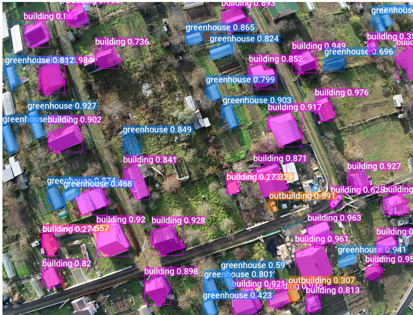
FIGURE 14. Results of detecting objects of different types using YOLO
