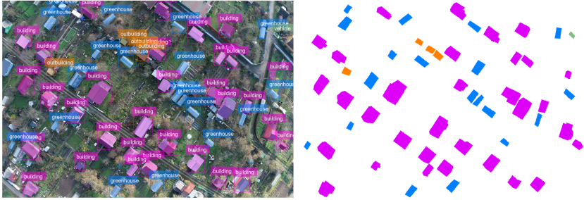
FIGURE 14. Swin-T (contour detection error \sim 3\text{--}5\% )
