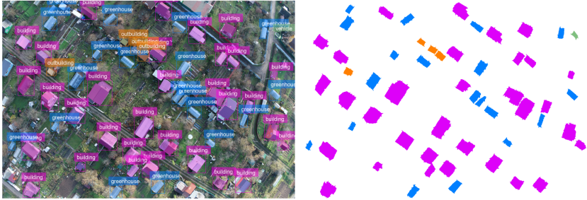
FIGURE 9. ResNet-50 (contour detection error \sim 15\% )
