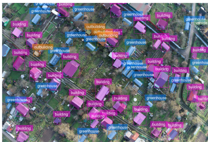
FIGURE 11. DenseNet-121 (contour detection error \sim 12\% )
