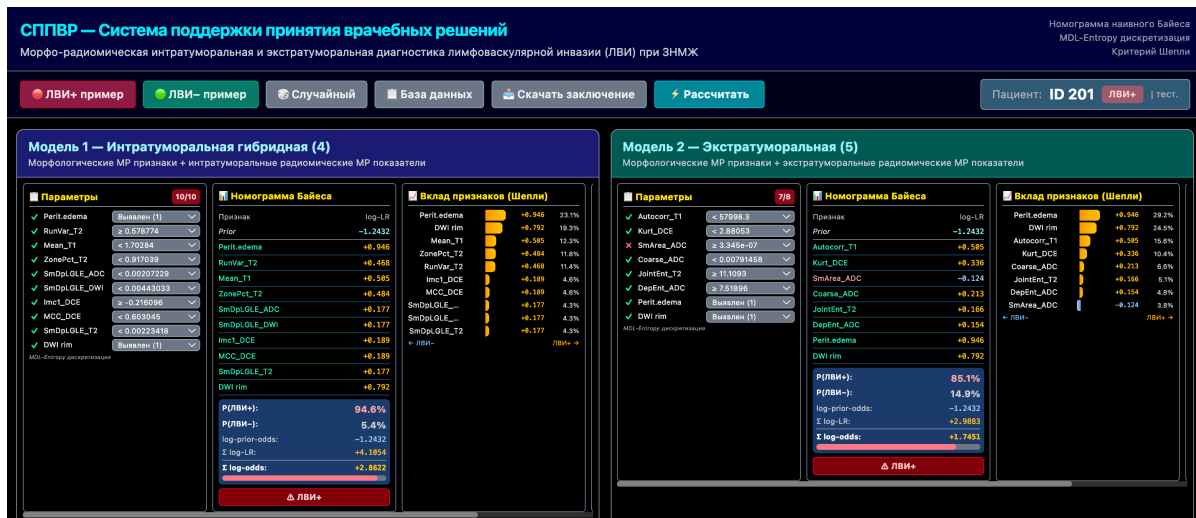
FIGURE 2. User interface of the "Morpho-radiomic diagnostics of LVI in MBN" CDSS prototype. Intratumoral panel is shown on the left, extratumoral panel on the right. The application is built as a standalone web tool running naive Bayes classification with Laplace smoothing ( \alpha = 1 ), Entropy-MDL binning, and integrated Shapley score / log-likelihood ratio calculations.
